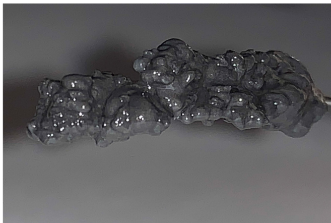
Figure 3 Photograph showing the lava-like formation of Menox cast being injected through a microcatheter in 0.9% NaCl suspension. The polymer solidifies centripetally in one solid mass.
