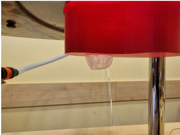
Fig. 4 Mesh shifting toward the hernial orifices which was considered recurrence
